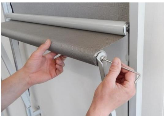
3. Make one turn of the bottom bar to roll the fabric and screw the movable part of the arm to the sides of the bottom bar.
